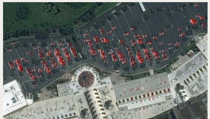
In this WorldView-3 image of the Westfield Brandon Mall near Tampa, Florida, AI-created bounding boxes highlight where cars are detected.
