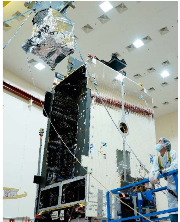
THE TEMPO PAYLOAD BEING LOWERED ONTO THE IS-40E SATELLITE.
